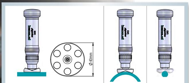
The optionally available special foot increases the measurement repeatability. It can be used for flat or curved surfaces. For curved surfaces there are two different apertures, one for diameters from 5 to 25 mm and one for larger diameters from 20 to 70 mm.
