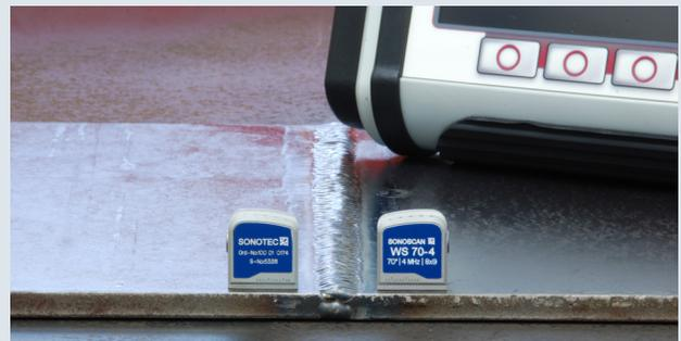
Ultrasonic angle beam probes (WS 45-4)
