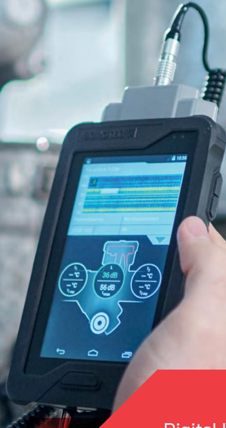
Digital Ultrasonic Testing Device
