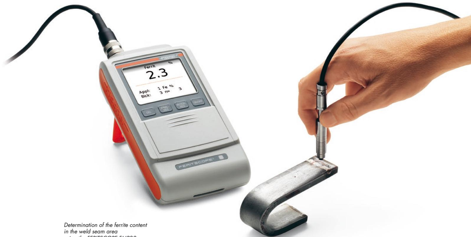
*Determination of the ferrite content in the weld seam area using the FERITSCOPE FMP30*
